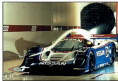
Use of smoke trace for off-body flow visualization in the wind tunnel test section.
